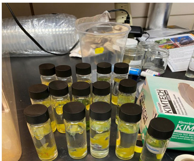
Figure 2: Prepared Experimental Vials. There are five vials for each tested groups (control-control, control-plastic, plastic-plastic) lined vertically.
